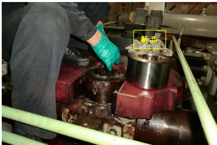
Tiller(舵柄) Roller bearing Ram pin Ram pin bush Ram(撞柱)
